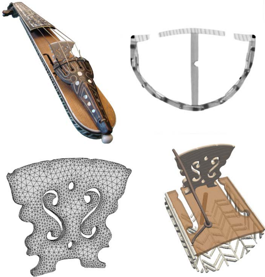
Fig. 1: Exemplary results of the proposed workflow (clockwise): photo of the kit violin, cross-sectional CT image (inverted grey values), rendering of segmented sub-structures, finite element model from surface data of the bridge.
